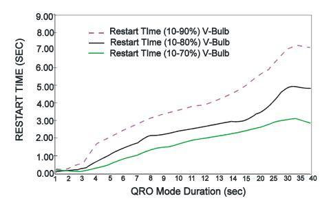
Figure 18. Restart Time Versus QRO State Duration, V-bulb
